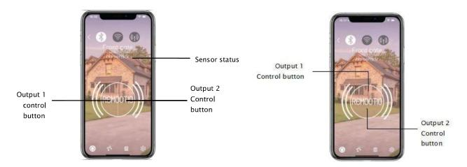
3. For Latching press and hold the output button and select the time period to hold output active
