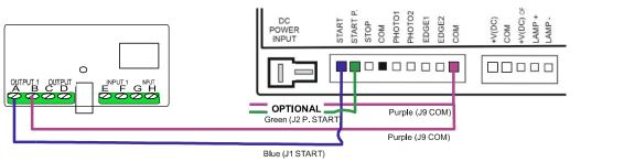
\* Optional connection determines the ability to toggle pedestrian function
